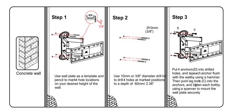
1. Level the wall plate to make sure the plate is centered on the back of the TV before marking the holes.
